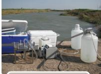
Large-volume suspended-sediment (LVSS) sampling equipment
