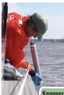
Kemmerer (depth specific) water-quality sampling
